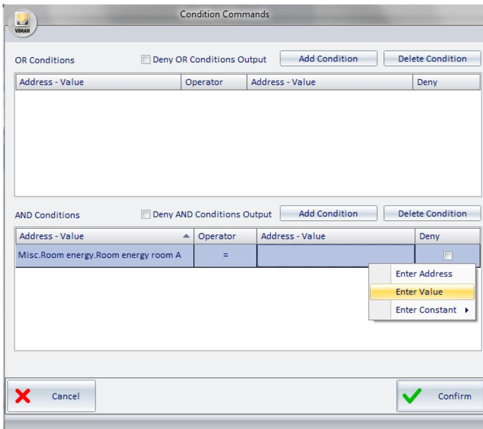
The screenshot shows the 'Condition Commands' dialog box with the 'AND Conditions' section active. The right 'Address - Value' field is selected, and a context menu is open over it, showing options: 'Enter Address', 'Enter Value', and 'Enter Constant'. The 'Enter Value' option is highlighted.
