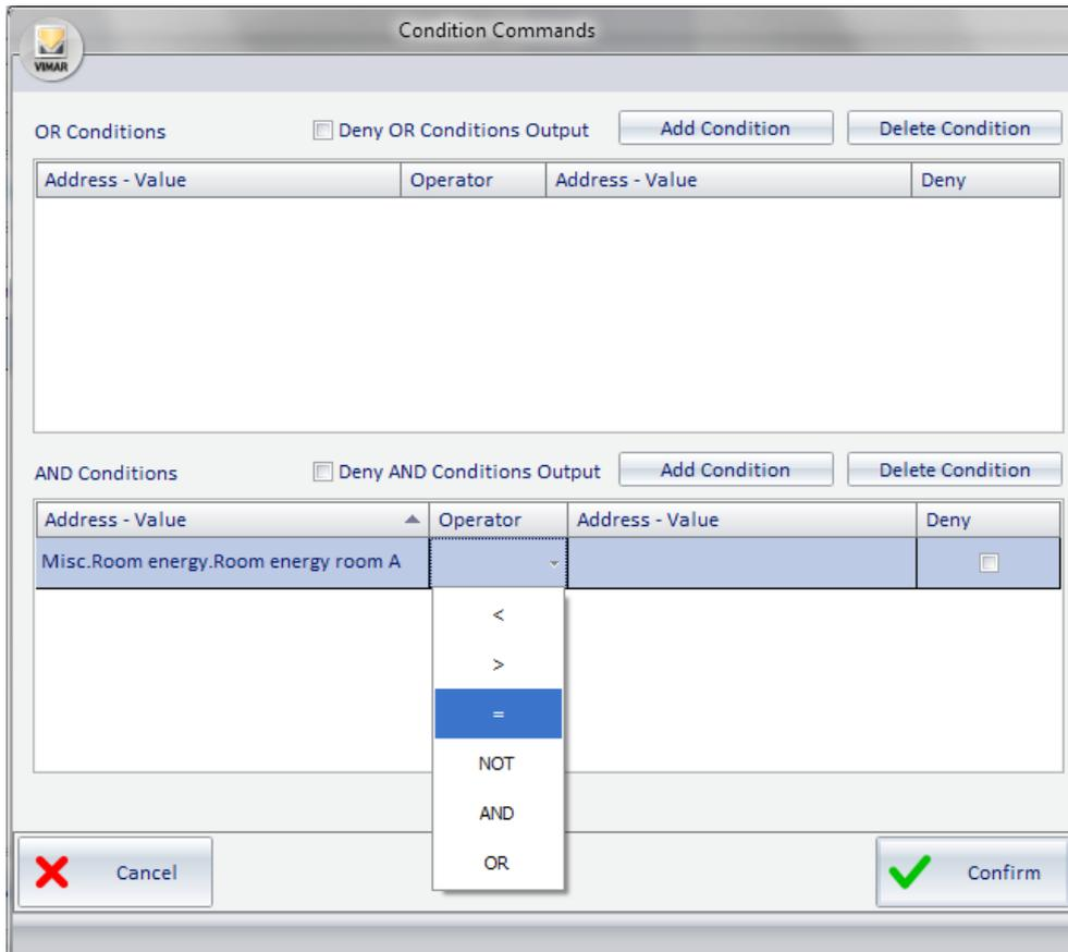
The screenshot shows the 'Condition Commands' dialog box with the 'AND Conditions' section active. A dropdown menu is open over the 'Operator' column, showing options: '<', '>', '=', 'NOT', 'AND', and 'OR'. The '=' operator is selected.
