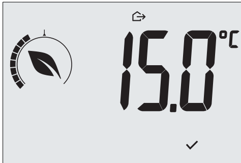
Fig. 11: Input in away mode showing the away temperature
