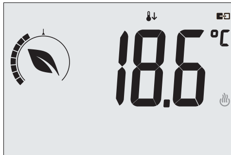
Fig. 16: Input in Remote reduction mode
