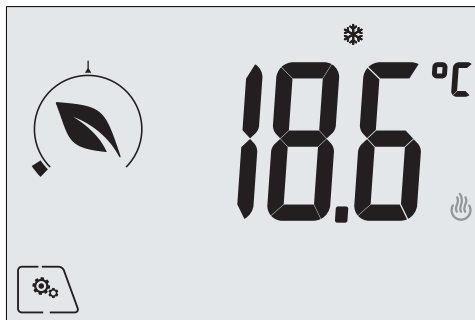
Fig. 14: Nighttime reduction mode
