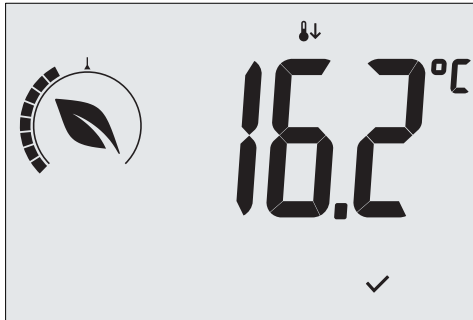
Fig. 14: Input in Nighttime Reduction mode showing the reduction set point
