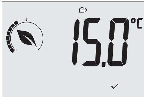
Fig. 12: Input in away mode showing the away temperature
