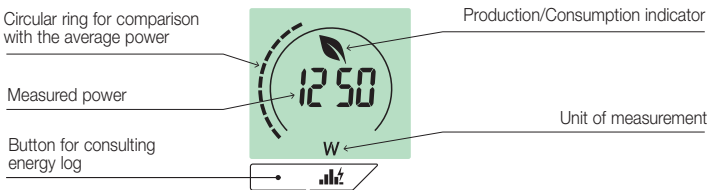
Fig. 5: Typical screen for consulting the energy probe
