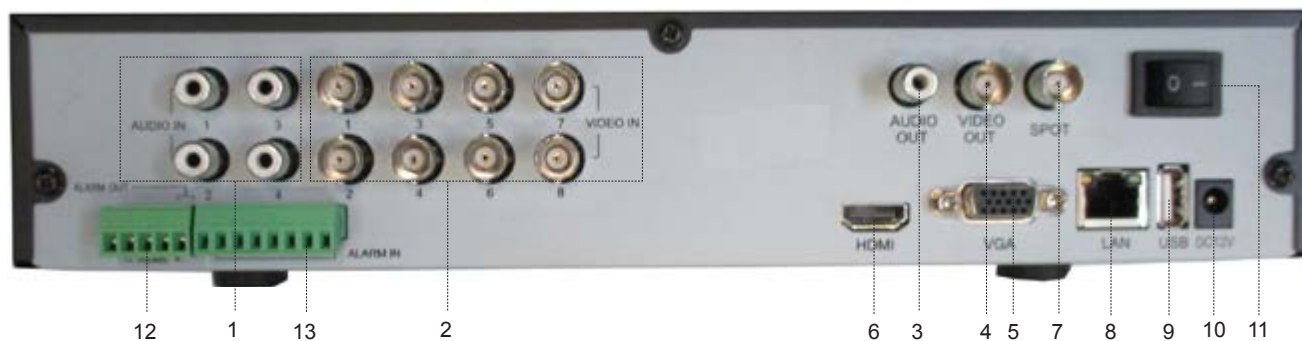
Fig 2-2 Rear Panel for 8-ch
