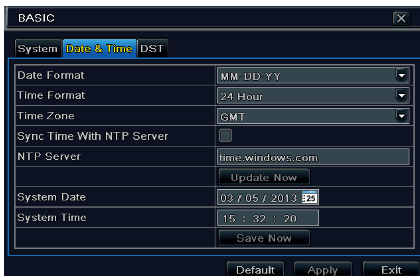
Fig 4-4 Basic Configuration-Date & Time
