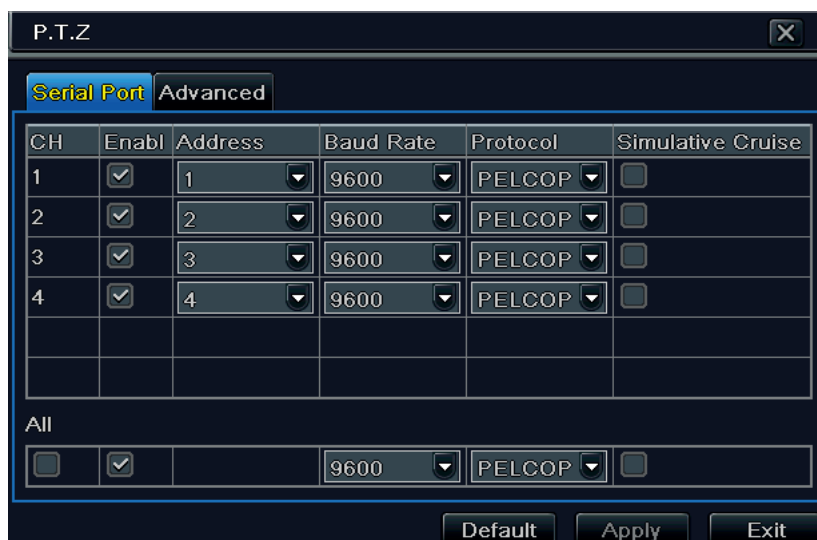
Fig 4-32 P.T.Z Configuration-Serial Port
