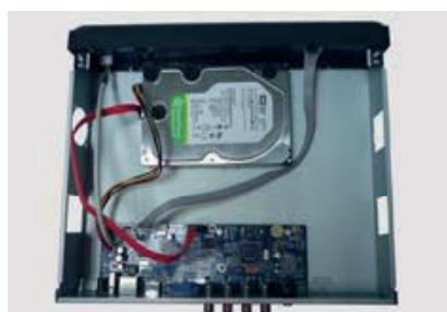
5. Connect the power and data cables.
