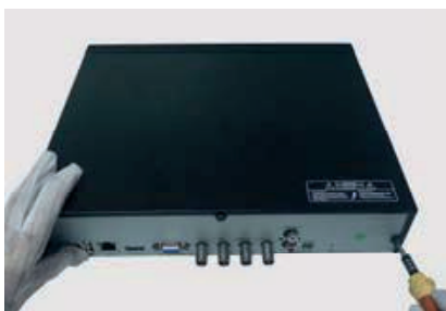
1. Loosen the screws on the back and side
