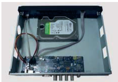
3. Put the HDD on the bottom of the device.
