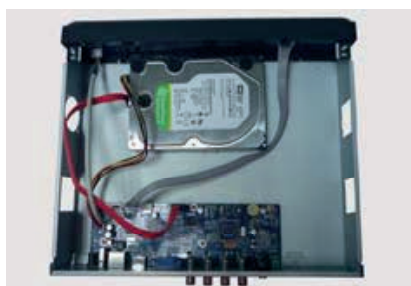
5. Connect the power and data cables.
