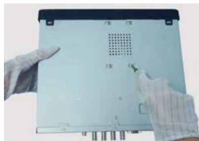
4. Turn over the device and fix the HDD with the screws.
