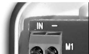
IN: input 1 of the external magnetic contact (configurable as normally closed or open).
